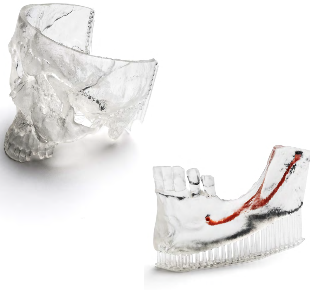
The 3D reproduction of a skull in which size, precision and transparency can be observed. Study models provide a view of the position of the patient's nerves, which is fundamental when studying and planning surgical actions.
